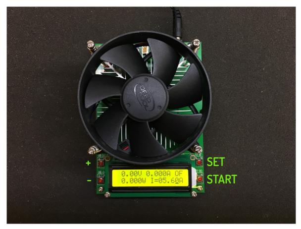
First of all please take note this load is not capable of 150W continuous dissipation and the voltage/current reading precision is not as good as specified as shown in my review video Voltlog #108.
